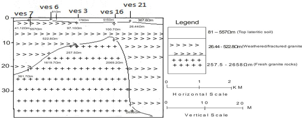
Fig. 4: Geo-electric section along profile AA' (VES 7, 6, 3, 16 and 21)
