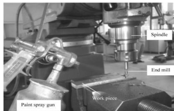
Fig. 1: Milling process under MQL (Duchosal *et al.*, 2013)
