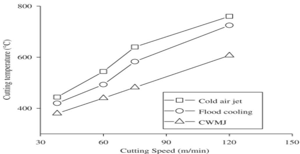
Fig. 2: Cutting temperature under different conditions (An *et al.*, 2011)
