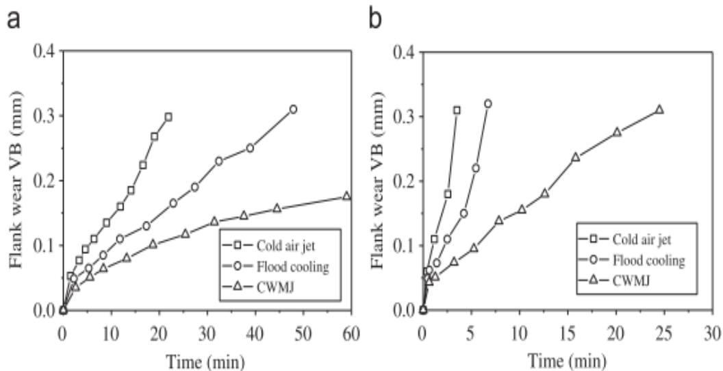
Fig. 3: Flank wear curves of cutting inserts under different cooling conditions, cutting Speed,  $V_c =$  (a) 38 m/min (b) 120 m/min (An *et al.*, 2011)
