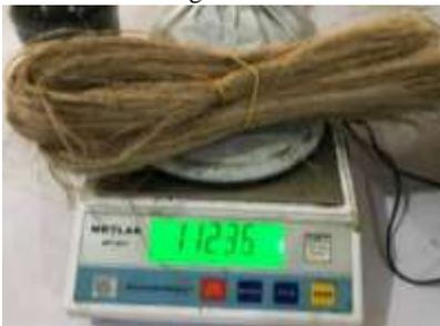
Plate VII: Weighed portion of the dried fibre.
